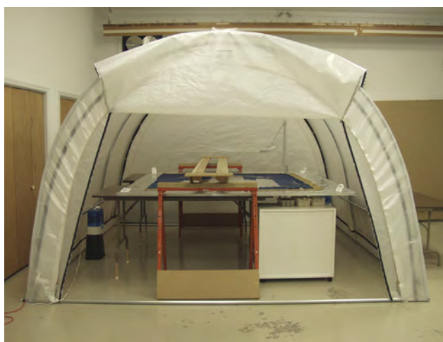
Figure 3. Humidification chamber with bridge and table. Photo courtesy of the author.
