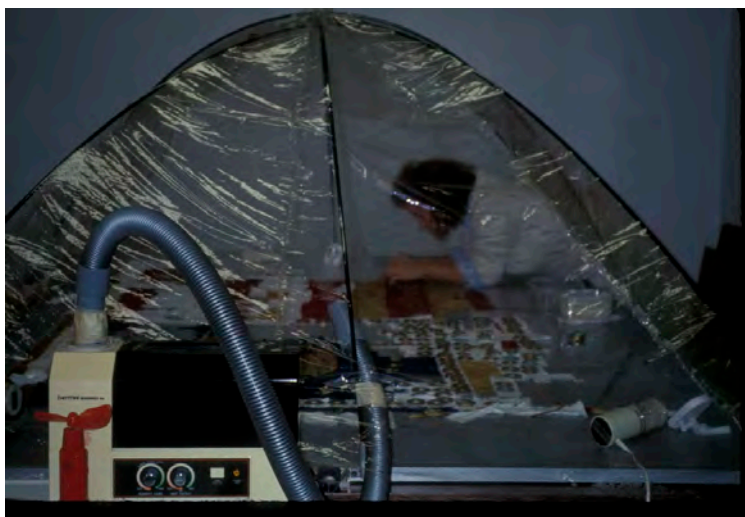
Figure 2. Table-top humidification set-up. Photo courtesy of the author.
