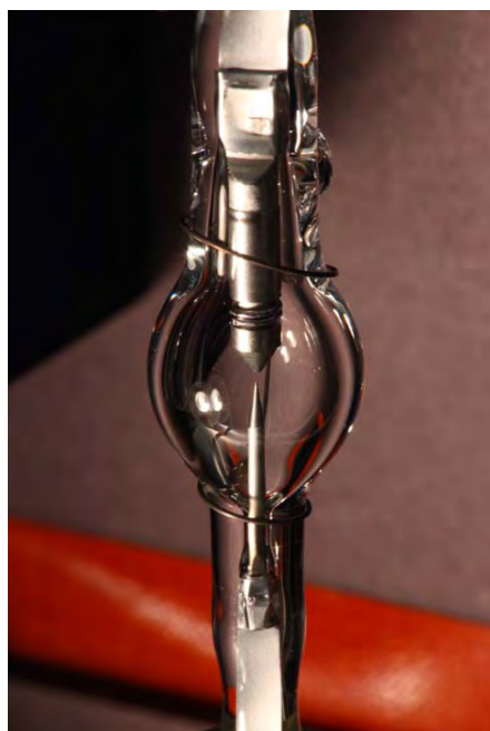
Figure 2 (left). 75 watt xenon lamp. Figure 3 (right). The xenon lamp housing with filter assembly (left tube assembly). The right side tube terminates with a photodiode array detector used to provide feed-back luminosity to the power supply.
