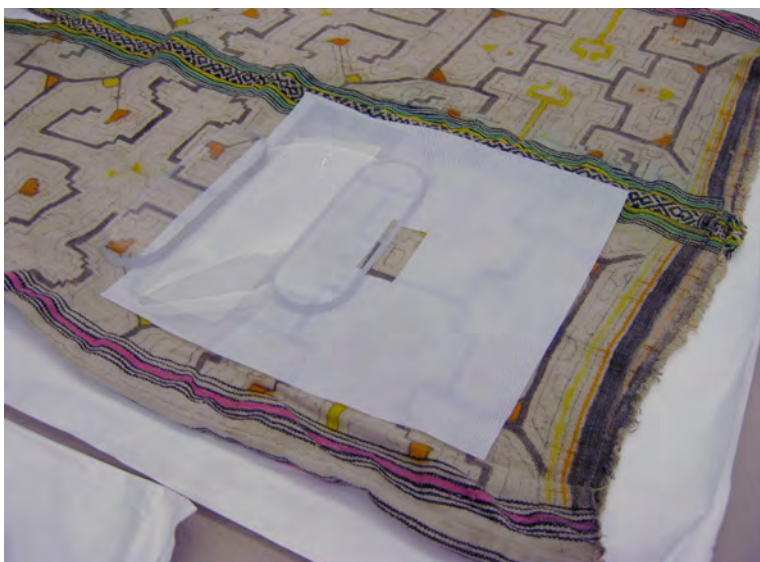
Figure 5. Contact humidification for crease removal during breathability testing using GoreTex® (left) and sample over a Shipibo cotton shirt. © NMAI.
