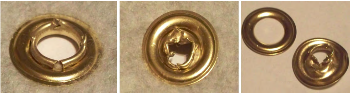
Figure 3. Steps of grommet removal showing snipped flange, pinched flange, and removed grommet.
