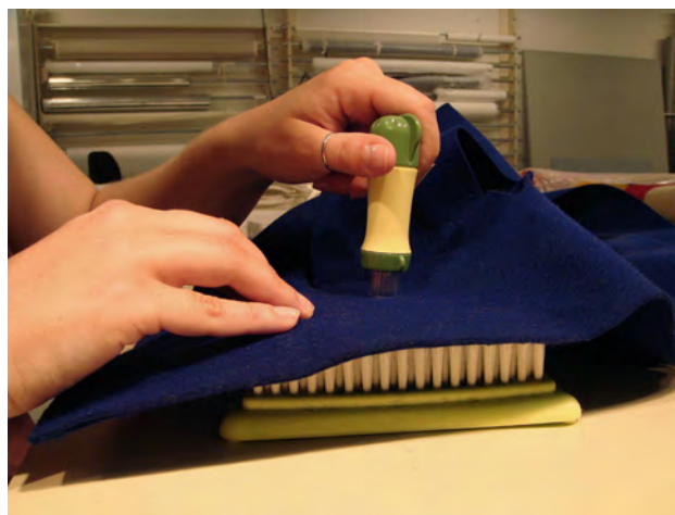
Figure 8. Needle felting process, showing felting punch and brush support.
