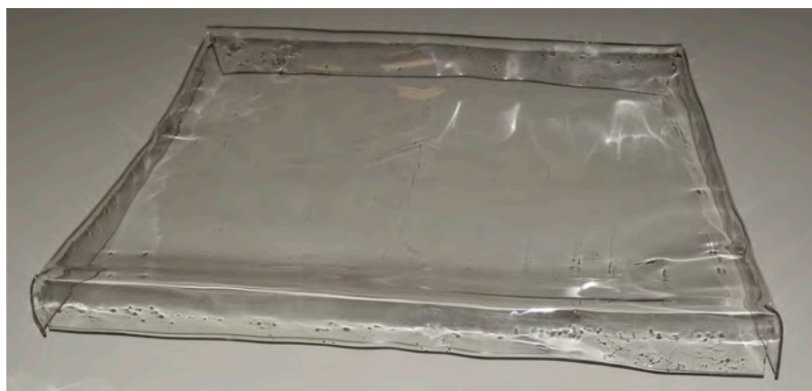
Figure 10. The upholstery support created through heat shaping.
