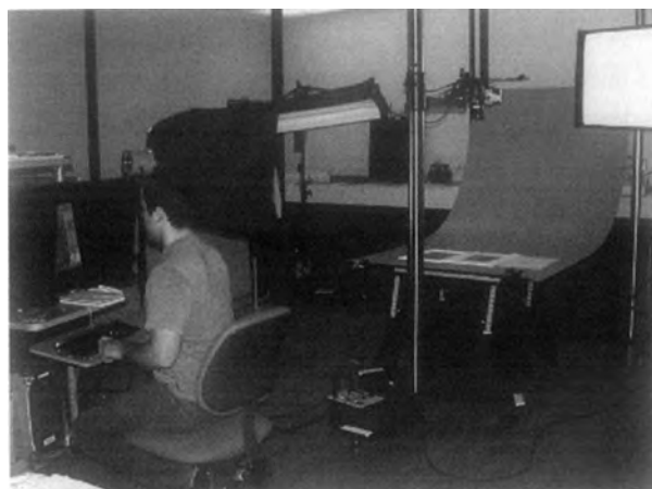
Figure 3. Nevamar is clamped to a tabletop and vertical poles to create a seamless backdrop for photography.
