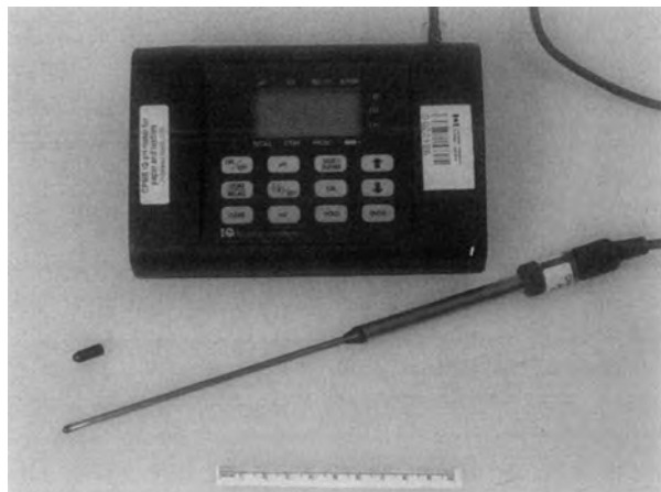
Figure 3. The IQ240 portable pH meter with micro probe. The cap has been removed from the tip of the micro probe.
